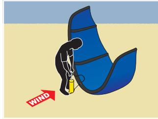
Make sure the clips on the air ducts leading to the struts are all open. Start pumping until the leading edge feels firm. If you prefer to use a pressure gauge, pump until it reaches about 6 psi.
